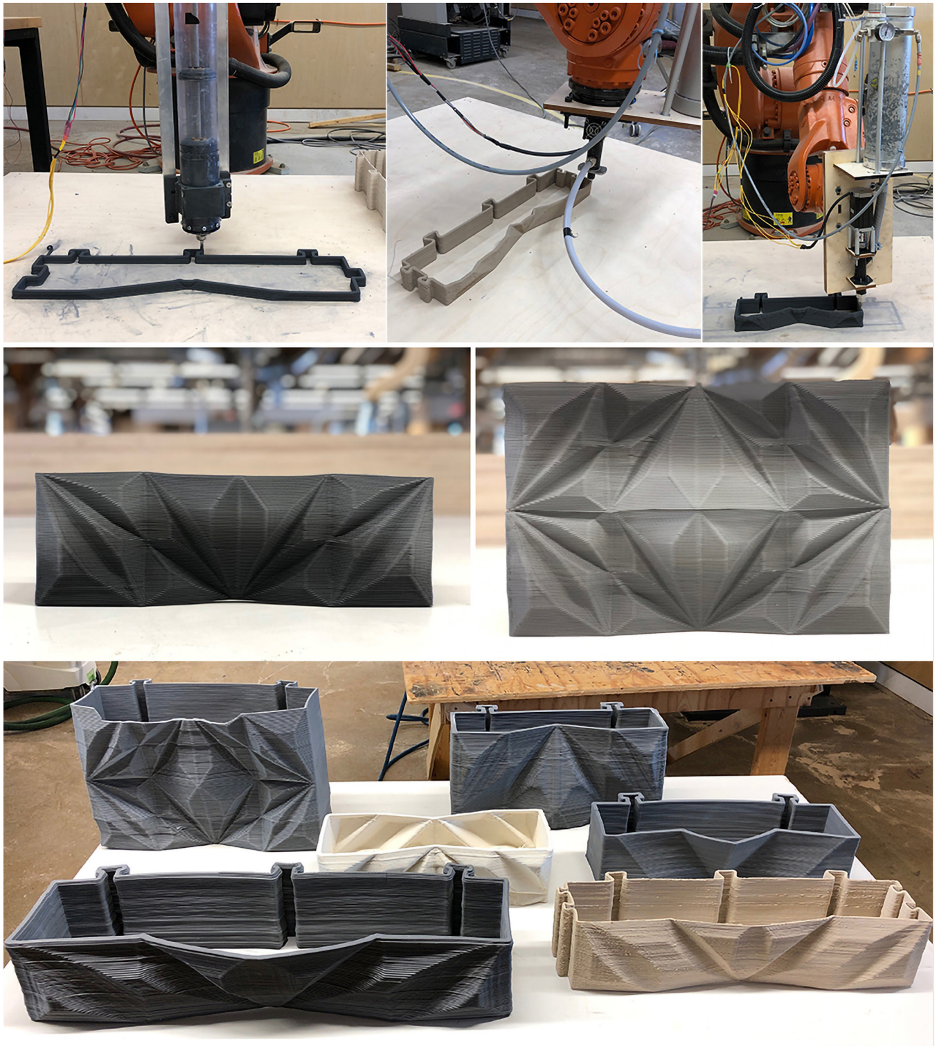
Figure 2. Ceramic prototypes exploring extruder, material and design limitations. Image by author.
