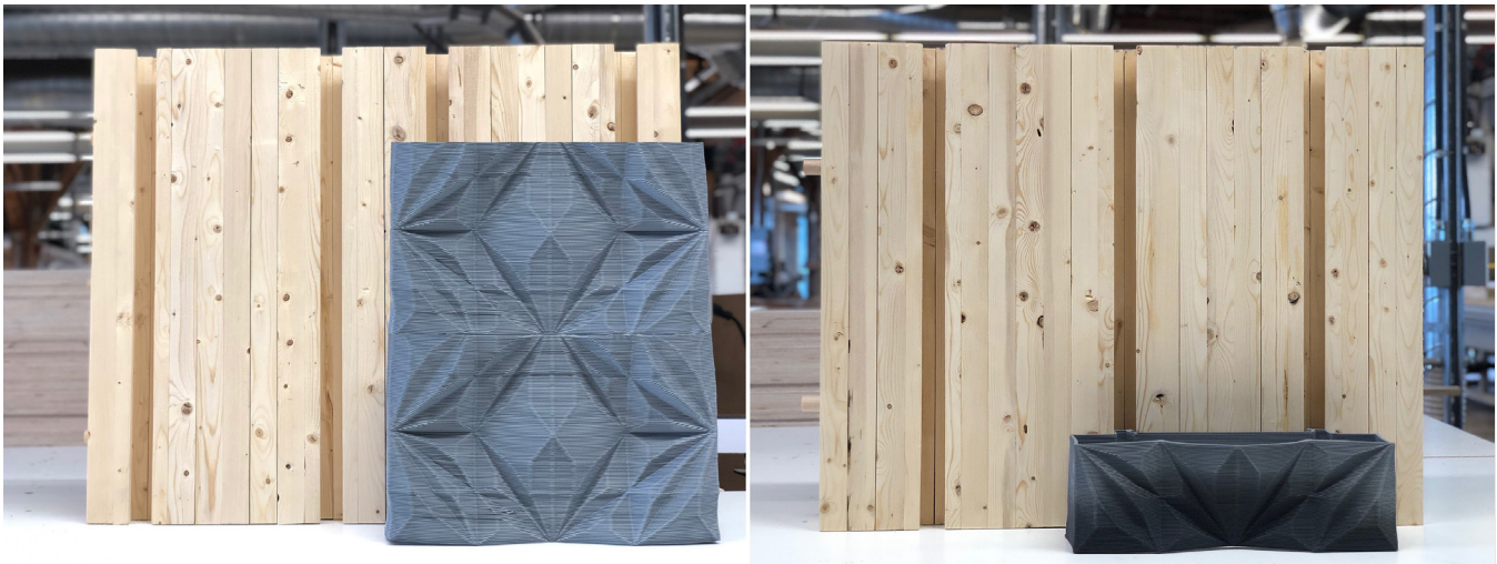
Figure 5. Work-in-progress prototype of a DLT-ceramic composite wall assembly. Image by author.
